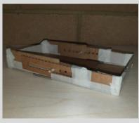
This is the first initial model of my finalised design and as you can see I have introduced the mechanisms that will be used within the assembly. I manufactured this design model using a CAD software programme called 2D Design that allows you to create a net of a design or the different components that will be used. This was then transferred to a laser cutter that cut out the separate components of my design in cardboard before printing my final product in acrylic sheeting.
