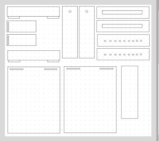
Here I have created a model of my final initial design using cad and 2D design. This is the net plan of my final packaging product. The whole design can be disassembled so that I can be sent back to the provider so that It can be used again for another customer to cut down on packaging waste and decrease profits that are used to contribute to the manufacture of this packaging.
